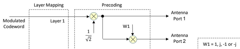
Figure 392 – Single layer precoding applicable when CSI Reference Signal uses antenna ports 3000 and 3001
