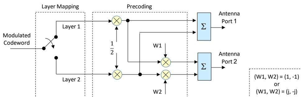
Figure 393 – Dual layer precoding applicable when CSI Reference Signal uses antenna ports 3000 and 3001
